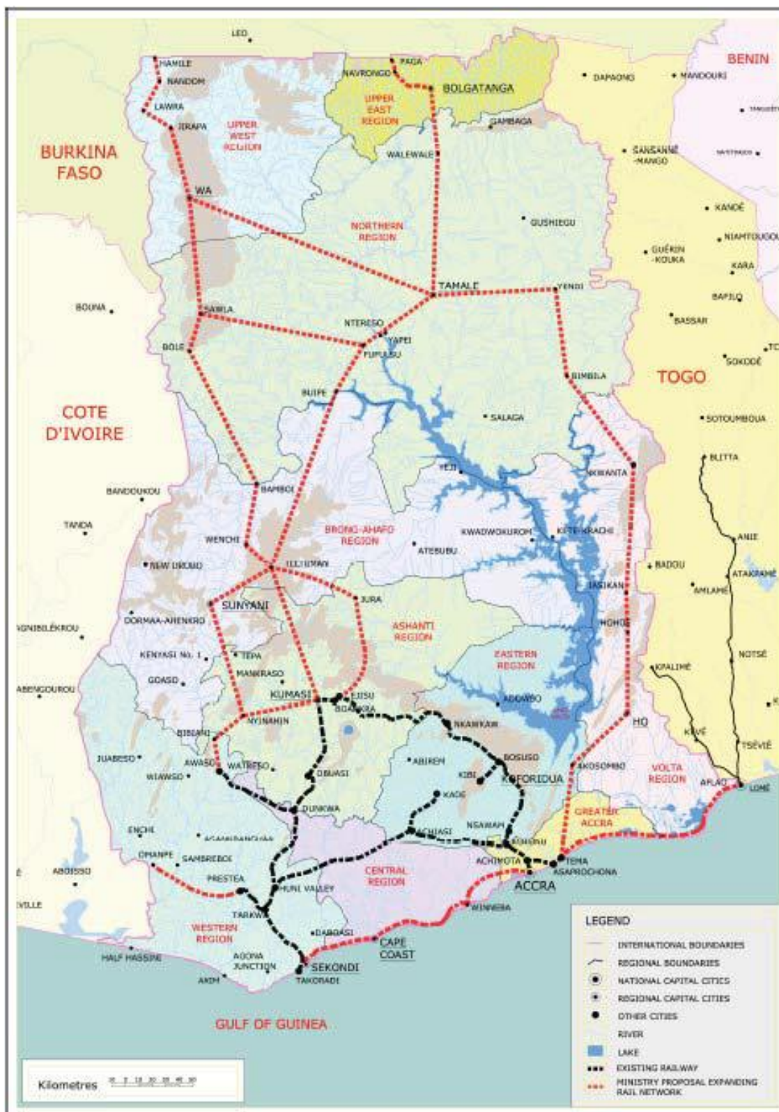
Fig. 2: Various options of Railway Line Extensions studied in the Ghana Railways Master Plan
